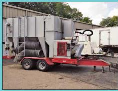
20,000 CFM Eagle Industries Model Jet-Clean 20-D Trailer Mounted 22-Cartridge Dust Collector
