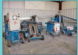
U.S. Filter Model "Porta Wheel" Vertical Shot Blast Cleaning System & U.S. Filter Blastrac 10DS Portable Floor Shot Blast Machine
