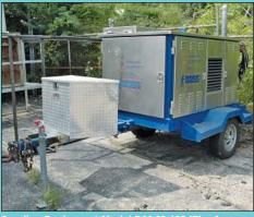
Carolina Equipment Model D44 60-100 "The Aqua Miser" Trailer Mounted Bicarbonate of Soda Stripper
