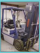
4500 Lb Komatsu Model FG 25ST11 Solid Tire LP Lift Truck
