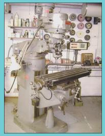
2 HP Bridgeport Variable Speed Milling Machine
