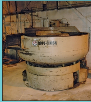
78" Roto-Finish Model Extended Range Spiratron Model ER-2530MS Vibratory Finishing Bowl
