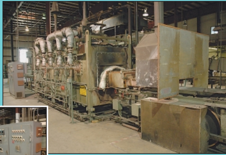
(2) 22" Wide Surface Combustion Model CBF-18-144 Natural Gas Fired Mesh Belt Atmospheric Brazing Furnaces
