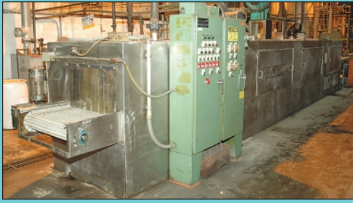
30" AFI Automated Finishing Inc. Natural Gas Fired Stainless Mesh Belt Parts Washer
