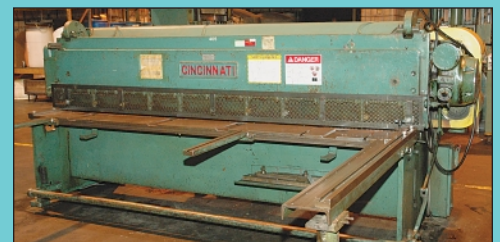
10 Ga. X 10' Cincinnati Model 1010 Mechanical Power Squaring Shear
