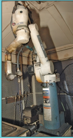
OTC Model IRB-481 Six-Axis CNC Two-Station Welding Robot
