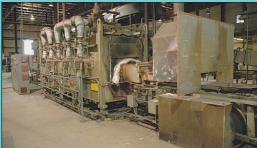
(2) 22" Wide Surface Combustion Model CBF-18-144 Natural Gas Fired Mesh Belt Atmospheric Brazing Furnaces
