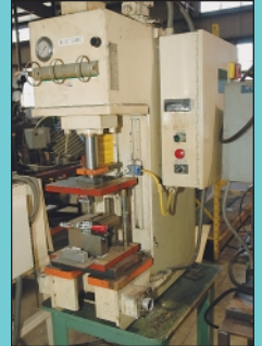
(2) 8 Ton PH Hydraulic Model PHN-8 Hydraulic Presses
