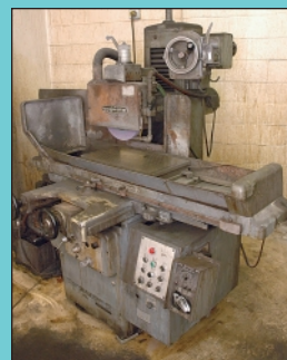
12" X 24" Okamoto Model Accugar 124 Hydraulic Surface Grinder
