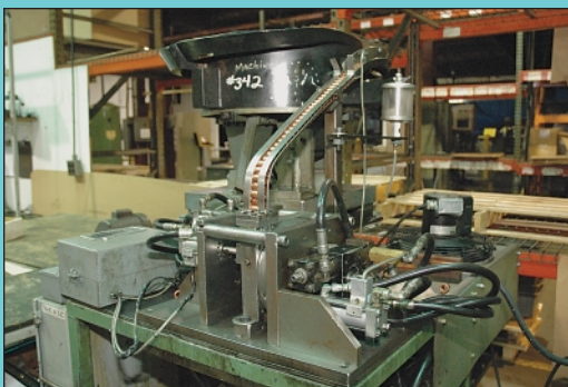
Mfg. Unknown Automatic Feed Tube End Coupling Former & Indent Machine
