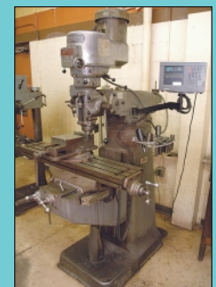
2 HP Bridgeport Series 2 Variable Speed Vertical Mill
