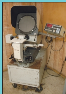
13" Mitutoyo Model PH-350 Optical Comparator
