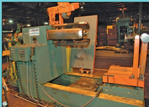
10,000 Lb. Dallas Model LC-1024 Hydraulic Uncoiler & w/ Coil Car
