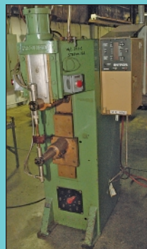
Partial View (1 of 4) Spot Welders To 150 KVA
