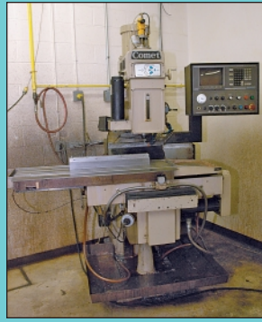
3 HP Comet Model 1632 D-20 CNC Vertical Milling Machine
