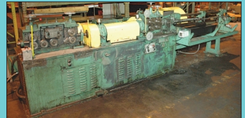
1/2" Schuster Model 3AV Automatic Wire Straightening & Cut-Off Machine
