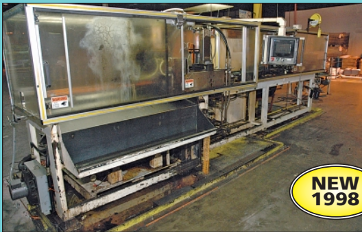
Crown Model STCOS-M10 Automatic Tube Straightening, Cut-Off & End Forming Machine
