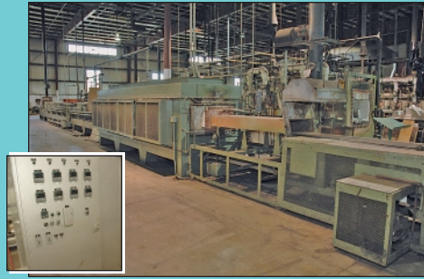
18" Wide Sargent & Wilbur Model CAC-1807-199 Electric Fired Mesh Belt Brazing Furnace
