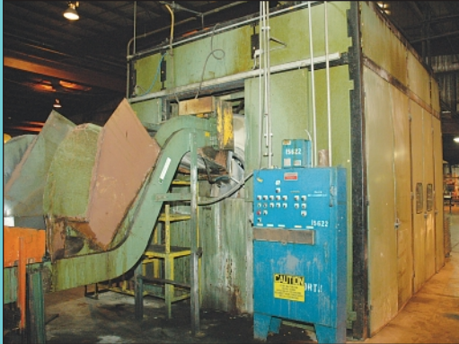
72" Dia. Ransohoff Model ELY15-622 Steam Fired Tumbling Drum Washer
