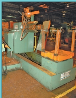
10,000 Lb. Dallas Model DPRL-1024-LH Uncoiler w/ Coil Car
