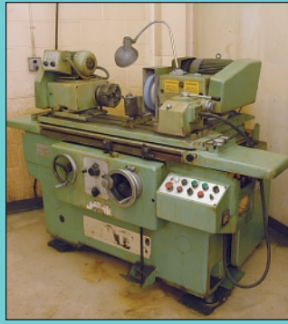
10" X 16" Shanghai Machine Tool Works Type MMB-1420 Universal Cylindrical Grinder
