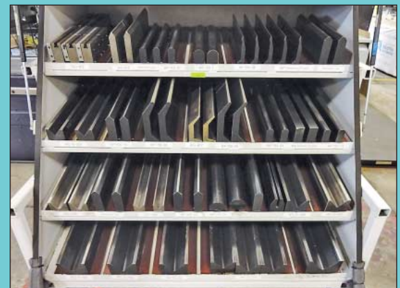
Large Quantity of Various Press Brake Dies by Wilson Tool and Wila
