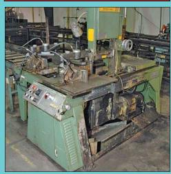
Marvel Model V-10A Tilt Frame Vertical Band Saw
