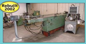
1-1/4" Pines Model No. 1 Horizontal Hydraulic Tube Bender
