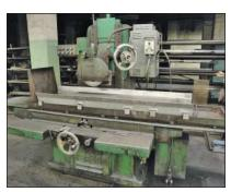
14" X 36" Gallmexer and Livingson No. 65A Hydraulic Surface Grinder w/ Electric Chuck
