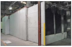
14' X 32' Approx. JR Greene Three-Pass Natural Gas Fired Combination Dry-Off and Cure Oven
