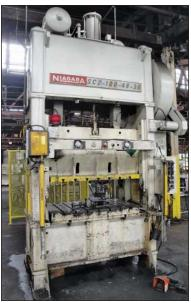
(2) 100 Ton Niagara Model SC2-100-48-30 Straight Side Double Crank Presses
