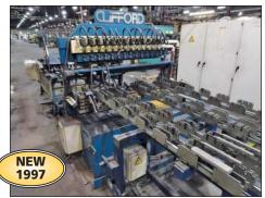
Clifford Model CWL EEZiWeld CNC Programmable Wire Mesh Welder
