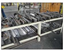
Partial View Large Quantity Press Brake Tooling
