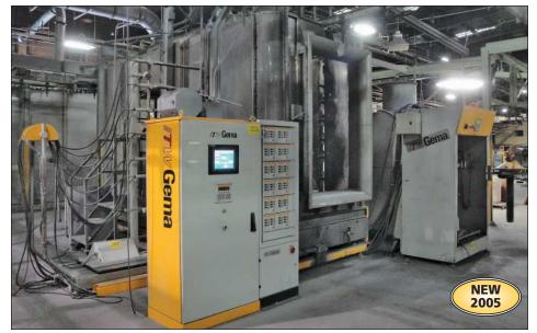
ITW Gema Optimatic 12-Gun Poly Upper Pass-Thru Automatic Powder Coat Booth
