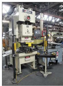
80 Ton Niagara Model Bison BN-80-OBS Variable Speed Gap Frame Press
