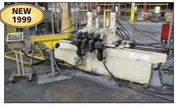
S&S FSD Model F50 Adjustable Dual Head Vertical Tube Bender
