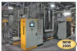
ITW Gema Optimatic 12-Gun Poly Upper Pass-Thru Automatic Powder Coat Booth
