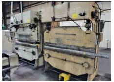
16 Ga. X 8' Diacro Hydra-Power Model 16-96 Mechanical Power Press Brake
