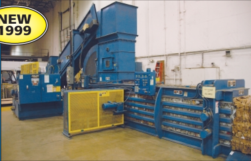
Harris / Selco Model HLO-128AT50-NB Open End Horizontal Hydraulic Baler w/ Auto-Tie – Jeffersonville Location
