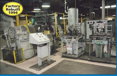
(5) 8,000 Ft. Lbs. Chambersburg Size 8MPC Impacter Horizontal Forging Machines
