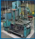
18" Marvel Model 81/M3M/M5/M6 Tilt Frame Vertical Band Saw
