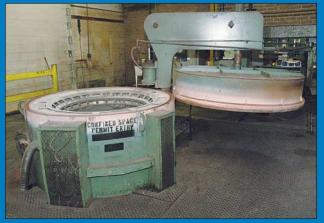
(4) 1,750 Degree Lindberg Model 12-R0-3836-174 Electric Fired Pit Type Furnaces
