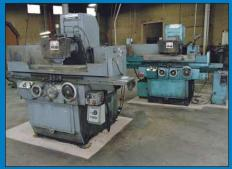
12" X 36" Brown & Sharpe Model 1236 Micromaster Hydraulic Surface Grinder
