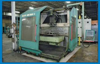
Maho Model MH1000S CNC Horizontal Machining Center
