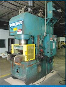
(2) 250 Ton Pacific Model 250 PFII Pressformer Hydraulic Cap Frame Presses
