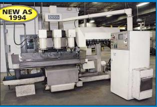
(2) Boston Digital Corp. Bostomatic 1000 Model 1741-3 Three-Spindle CNC Vertical Machining Centers
