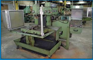
Maho Model MH-700C CNC Horizontal Machining Center
