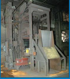
36" Dia. X 48" Wide Wheelabrator Tumblast Steel Belt Abrasive Blast Machine
