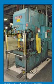
150 Ton Pacific Model 150 PFII Pressformer Hydraulic Gap Frame Press
