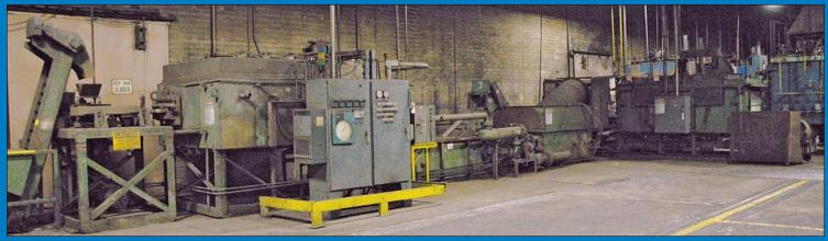
Overall View Sunbeam Shuffle Hearth Furnace Line w/ Annealing and Draw Furnaces, Quench Tank, Washer and Loader
