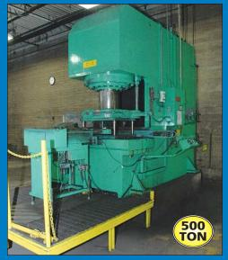
500 Ton Pacific Model 500 PFII Pressformer Hydraulic Gap Frame Press
