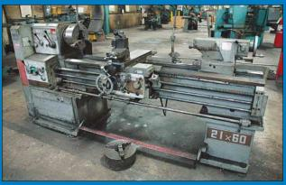
21" X 60" Kingston Model 2160 Geared Head Engine Lathe
