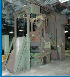
24" Dia. X 36" Wide Wheelabrator Tumblast Rubber Belt Abrasive Blast Machine
