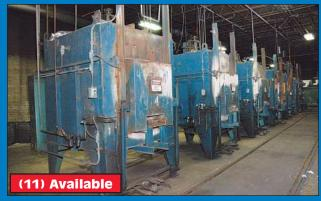
Overall View (11) Convection Tempering Furnaces By Surface Combustion and IFSI
