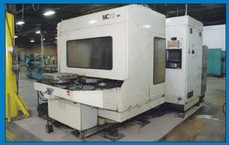
Leblond Makino Model MC65 Two-Pallet CNC Horizontal Machining Center
