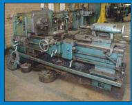
21-1/2" X 48" Cincinnati Tray-Top Geared Head Engine Lathe
