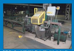
7/8" Bar Cap. X 12" Wide Blade Mfg. Unk. Hydraulic Alligator Style Shear  $\,$
