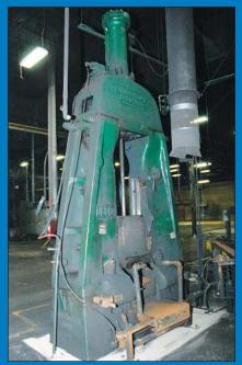
(2) 2,500 LB Chambersburg Ceco-Drop Model 25CD Forging Hammers
