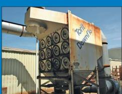
30 HP Torit Donaldson Downflo Model T3-24 Cartridge Type Dust Collector
