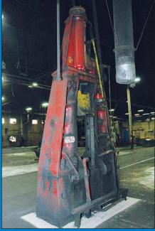
1,500 LB Chambersburg Model 15DHE Double Acting Dual Forging Hammer
