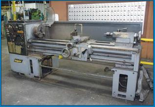
16" X 60" Bridgeport Romi Model 16-8 Geared Head Engine Lathe
