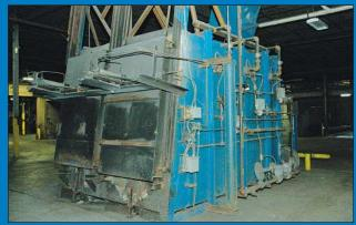
Air & Energy Systems Natural Gas Fired Dual Chamber Casting Pre-Heat Furnace
