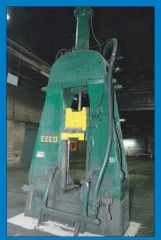
(4) 2,000 LB Chambersburg Ceco-Drop Model 20CD Forging Hammers
