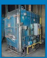
(4) Surface Combustion Electric Convection Tempering Furnaces
