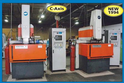
(2) Charmilles Model Roboform 40 Four-Axis CNC Die Sinker EDM's
