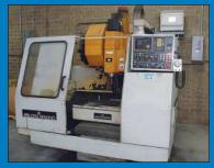
Makino Model FNC60 CNC Vertical Machining Center
