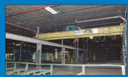
7-1/2 Ton X 35' Approx. Span Progressive Double Girder Top Running Overhead Bridge Crane
