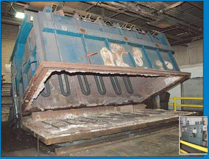
12' X 24' X 12'H Industrial Furnace Services Inc. Type Flip Up Natural Gas Fired Furnace
