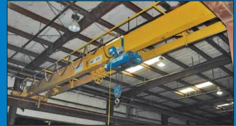
7-1/2 Ton X 40' Approx. Span Anchor Crane Overhead Crane System w/ 150' Free-Standing Crane Rail
