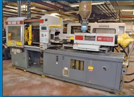
120 Ton X 8 Oz. Van Dorn Model 120-RS-8F-HT Toggle Clamp Plastic Injection Molding Machine
