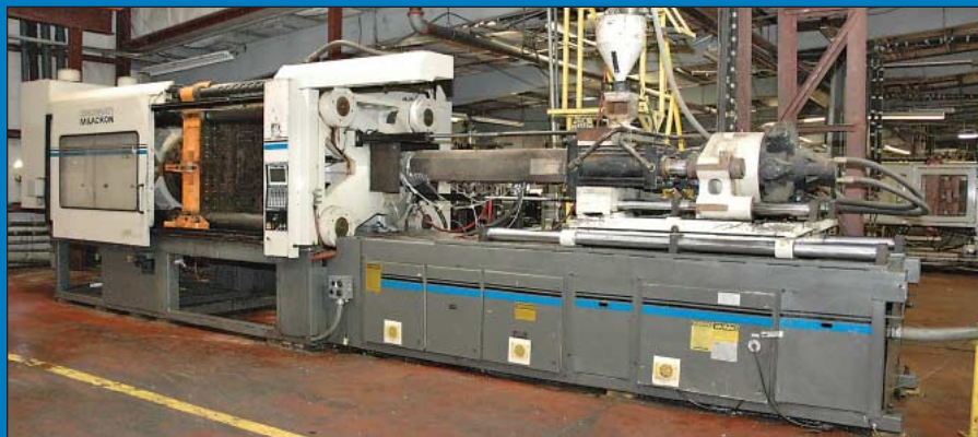
850 Ton X 140 Oz. Cincinnati Milacron Model VH850-140 Hydraulic Clamp Plastic Injection Molding Machine
