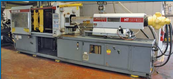
300 Ton X 30 Oz. Van Dorn Model 300-30FH Toggle Clamp Plastic Injection Molding Machine
