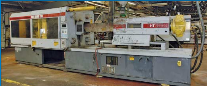
500 Ton X 60 Oz. Van Dorn Model 500HT-RS-60F Toggle Clamp Plastic Injection Molding Machine
