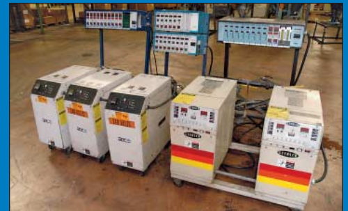
Partial View Thermolators and Hot Runner Controllers
