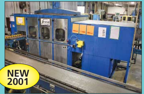
Jen Fab Automated Vertical Agitation Parts Washer w/ Ultrasonics
