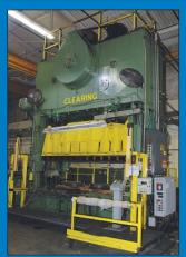
300 Ton CMC Clearing Model F-4300-148 SSDC Press
