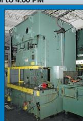
220 Ton Aida Model C2-20(2) Double Crank Gap Frame Press
