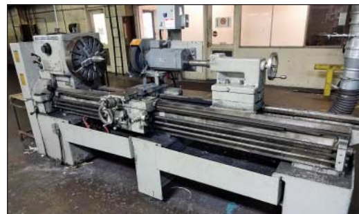
(15) Roller Lathes w/ Grinding, Sanding and Polishing Toolposts to 72" Swing and 240" Centers
