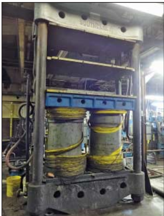
(30) 400 Ton to 7 Ton Compression Rubber Molding Presses w/ Bed Sizes from 42" x 42" to 12" x 12"
