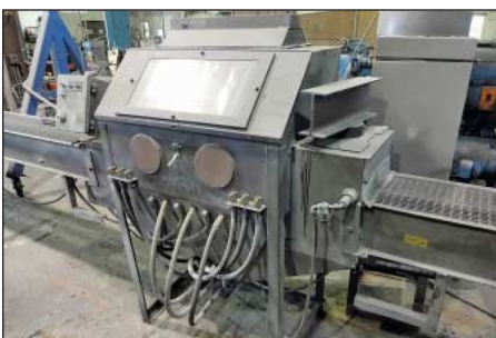
24" x 36" Econoline Blast Cabinet w/ 12" Belt Thru Feed Conveyor and Reclaim
