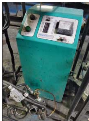
Prosco Model 200 Elastomer Cutting System w/ Electrically Heated Cutter
