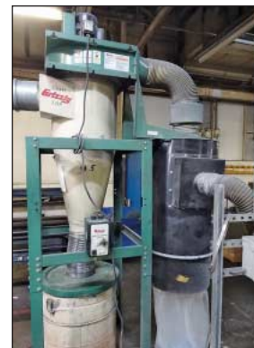
(5) 3 HP Grizzly Model G-0441 Cyclone Type Dust Collectors
