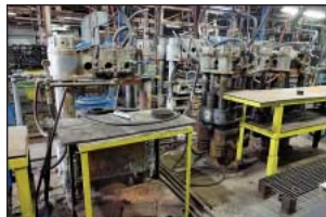
(30) 400 Ton to 7 Ton Compression Rubber Molding Presses w/ Bed Sizes from 42" x 42" to 12" x 12"
