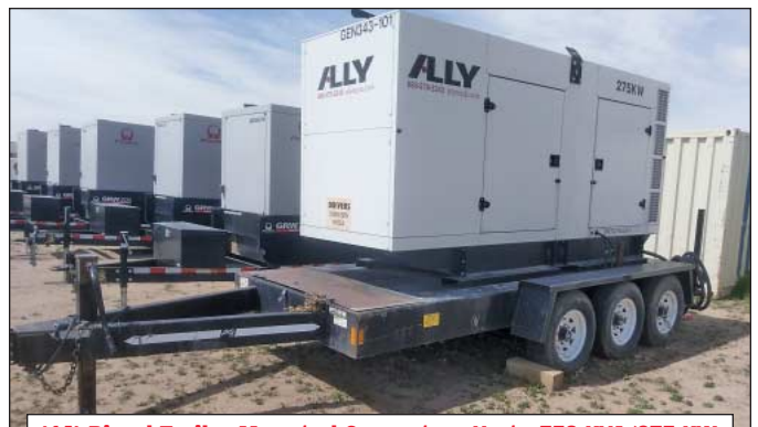
(14) Diesel Trailer Mounted Generators Up to 350 KVA/275 KW
