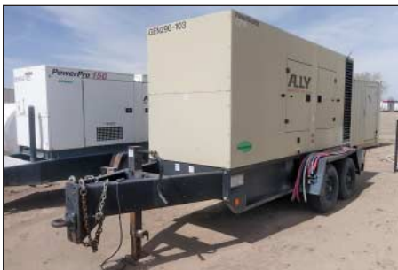
290 KVA / 232 KW Ingersoll Rand / Doosan Trailer Mounted Diesel Generator
