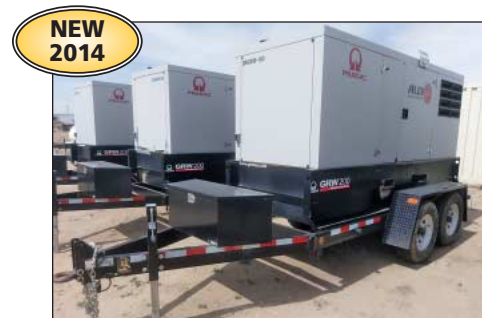
(5) 200 KVA / 160 KW Pramac Trailer Mounted Diesel Generators
