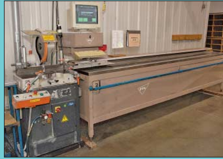
Overall View (4) 14" Elumatec Saws and (2) PTC Programmable Stops
