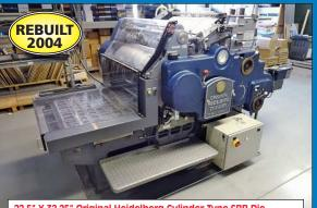
22.5" X 32.25" Original Heidelberg Cylinder Type SBB Die Cutting Press (Rebuilt 2004 By Whittenburg)
