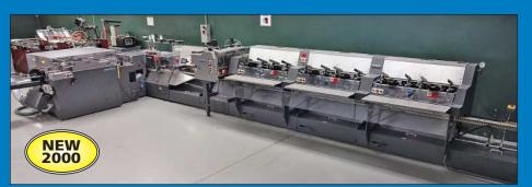
Heidelberg Prosetter Model SP455-S Six-Pocket Saddle Stitching Line w/ Three-Knife Trimmer
