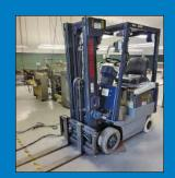
3,500 Lb. Komatsu Model FB18SH6 Electric Lift Truck
