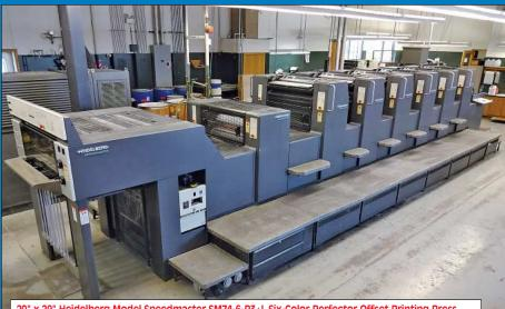
20" x 29" Heidelberg Model Speedmaster SM74-6-P3+L Six-Color Perfector Offset Printing Press w/Coating Tower
