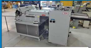
30" Rollem Model TR30 Die / Score System, Perforating /Scoring /Creasing /Slitting Machine
