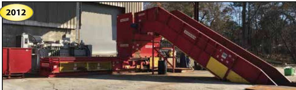
2012 SIERRA INTERNATIONAL MACHINERY REB-2 44" x 29" Scrap Baler w/2012 72" Wide Incline Feed Conveyor
