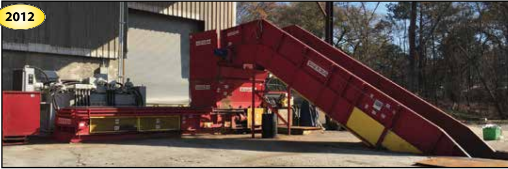
2012 SIERRA INTERNATIONAL MACHINERY REB-2 44" x 29" Scrap Baler w/2012 72" Wide Incline Feed Conveyor
