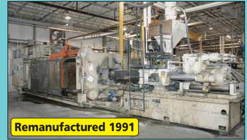
1,500 Ton X 225 Oz. Farrel / HPM Model RS225-1500 Hydraulic Clamp Injection Molding Machine
