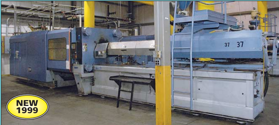
880 Ton X 160 Oz. HPM Model MLH880-160HP1 Hydraulic Clamp Injection Molding Machine
