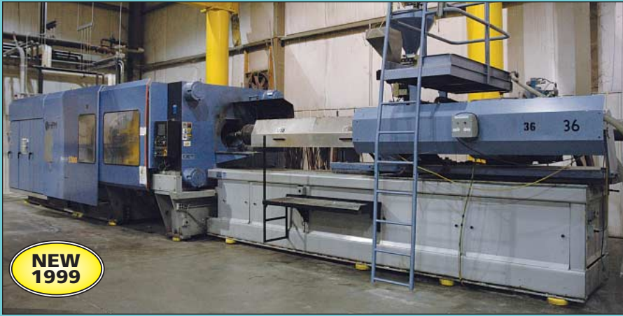
1,100 Ton X 191 Oz. HPM Model MLH1100WP Wide Platen Hydraulic Clamp Injection Molding Machine
