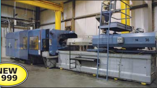
1,100 Ton X 191 Oz. HPM Model MLH1100WP Wide Platen Hydraulic Clamp Injection Molding Machine
