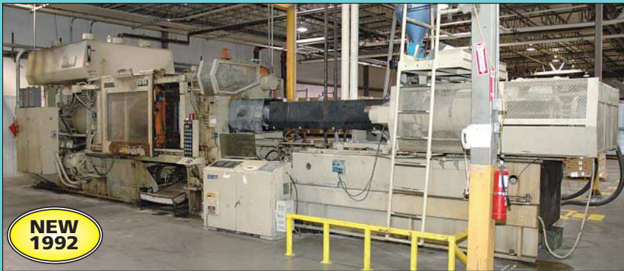
1,000 Ton X 260 Oz. HPM Model 1000-MK-II-260 Hydraulic Clamp Injection Molding Machine
