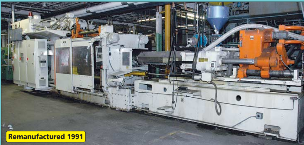
1,000 Ton X 140 Oz. HPM / Cincinnati Milacron Model 1000-IX-140 Hydraulic Clamp Injection Molding Machine
