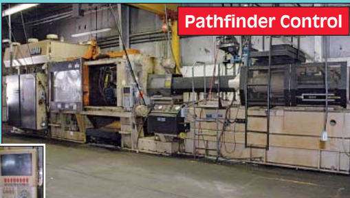
1,000 Ton X 160 Oz. HPM Model 1000-MKII-160 Hydraulic Clamp Injection Molding Machine
