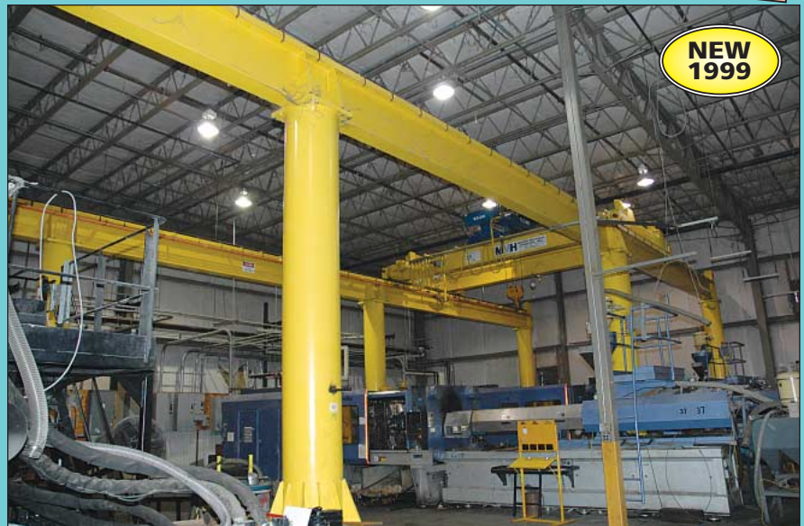
25 Ton X 25' Approx. Span X 120' Approx. Long Macko Material Handling Free-Standing Overhead Bridge Crane
