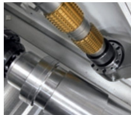
Tool combinations on one tool spindle Vibration-free steel-polymer structure Optimum chip flow and evacuation
