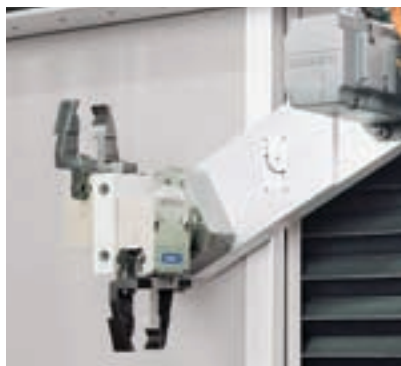
Gantry loader in light aluminium construction with swivelling gripper wrist.
