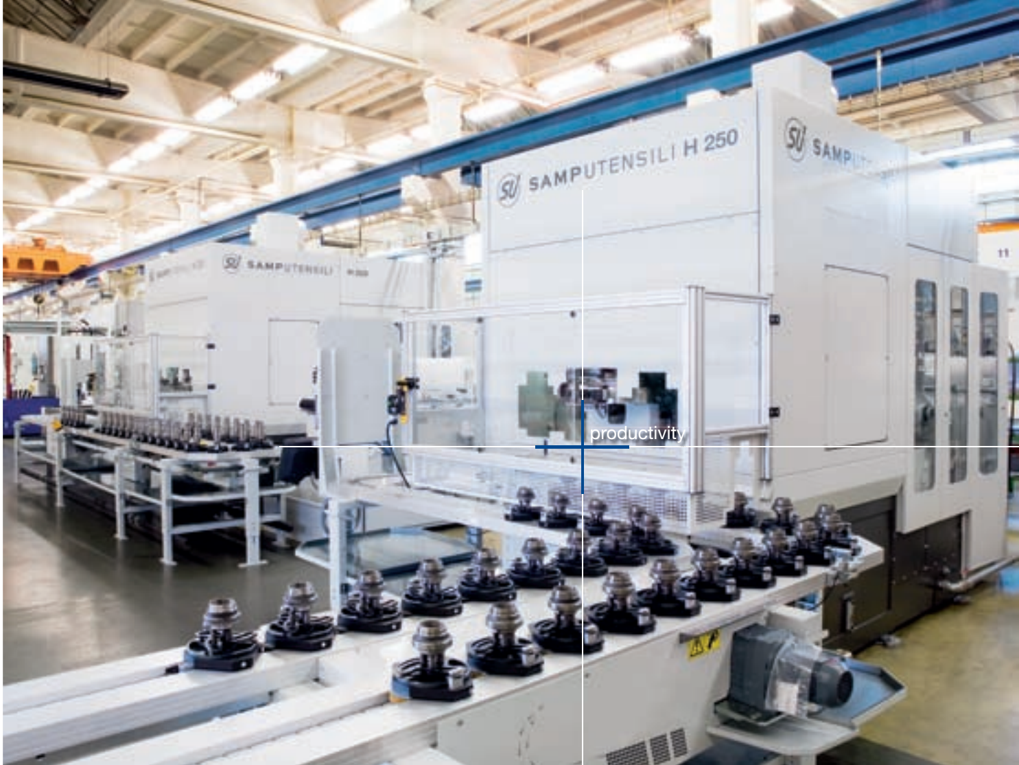
H 250 machines automated with ringloader and workpiece magazine with 50 stations.
