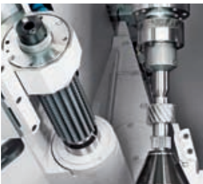
Hobbing with HSS hobs coated with new Sunite® Alcrona.
