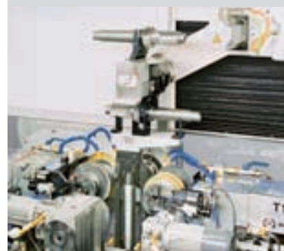
Chamfering/deburring unit with two self-centering tool heads for one tool group each
