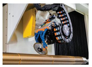
6-Axis design allows for (3) rotary motions and (3) linear motions and are simultaneously controlled allowing for the manufacturing and re-sharpening to today's most demanding designs.
