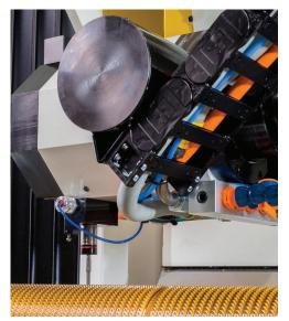
The dual probe system allows for a part probe to locate the cutting edges of the workpiece and reference it to the machine while the wheel probe (shown) locates the grinding wheel relative to the workpiece.
