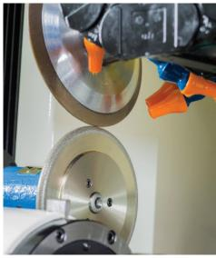
The wheel truing cycle is programmed into the machine. Simply enter the amount of stock removal and the machine automates the cycle.
