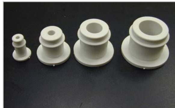
Representative "doodads" and "gadgets" used as chip defectors during the gundrilling operation. Available from Star SU.
