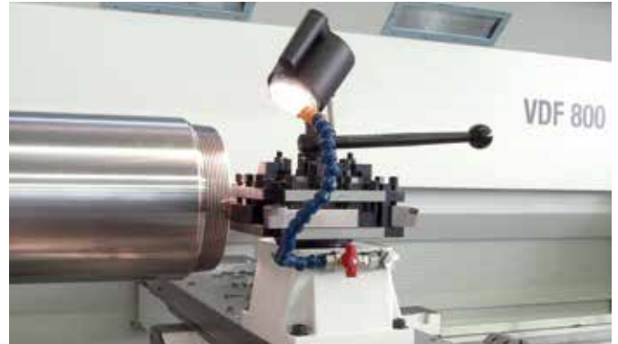
Re-cutting of threads on a VDF 800 DUS
