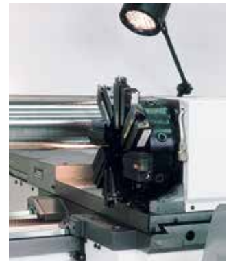
8-position disc turret, driven tools as option
