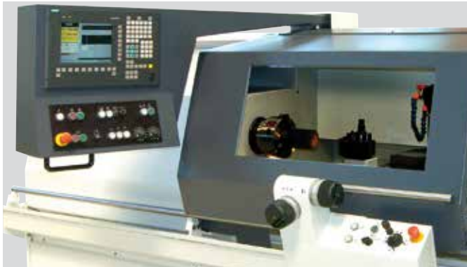
Pivoting control panel. Non-traveling chip protection door
