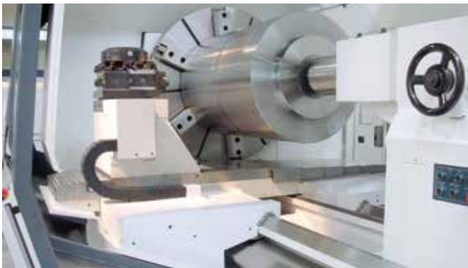
Work zone with 4-position universal turret
