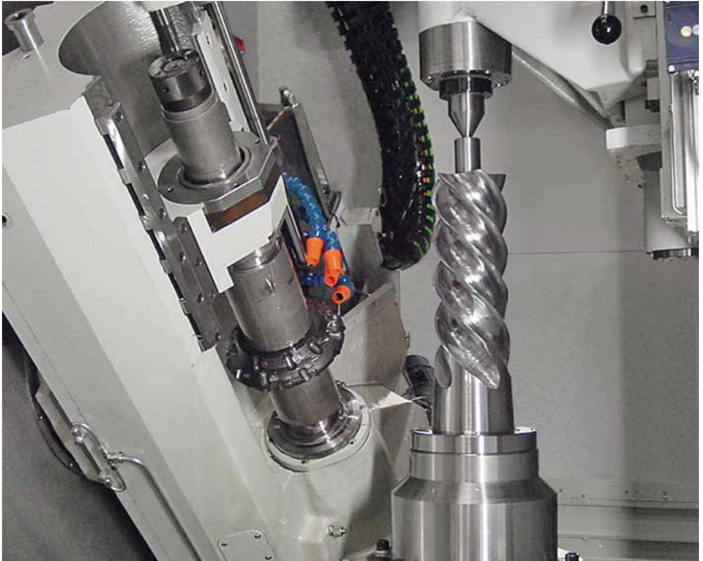
The H 600 equipped with PowerCutting options is especially suited for the milling or hobbing of large rotors
