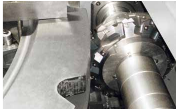
Form milling of large sprocket gears
