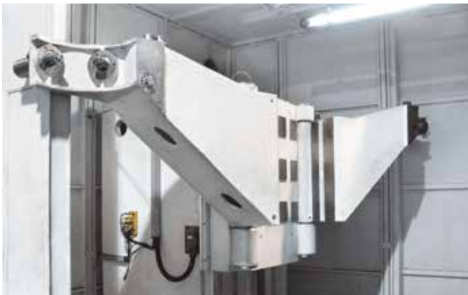
The smart swing-away tailstock arm can be opened completely to leave the workarea free for the workpiece change from above
