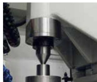
Automated tailstock with cam-free adjustment
